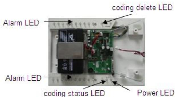
1. **Power LED** will be on when the siren is connected with external AC power;
